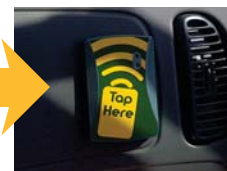
RFID reader captures student RFID Card Number
