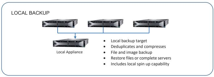
As an added feature and depending on the configuration ordered, the local appliance can act as a local disaster recovery system during a server level disaster scenario by spinning up a virtualized copy of one or more protected servers.
