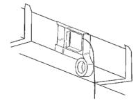
6. Unit may be taped with aluminum HVAC tape to provide complete seal.
