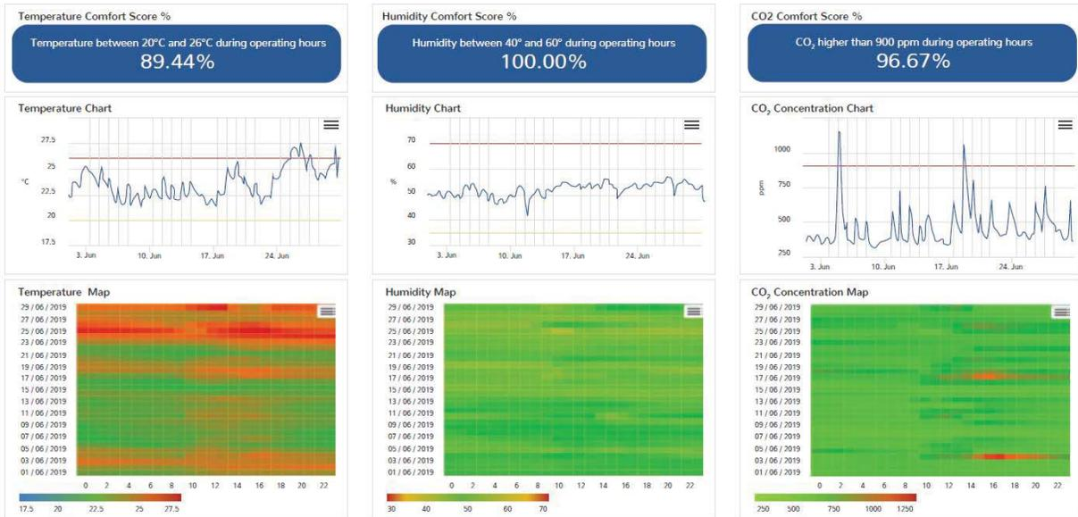
If parameters exceed thresholds, then the system produces alerts. Minimise' Internet of Things (IoT) and Artificial Intelligence (AI) technologies can make changes to the existing Building Management System (BMS) to correct any alerts. The system provides a twofold benefit:
