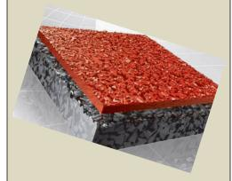
**DynaTrack-S2™:** A two layer, 13 mm, permeable spray coat track system. The base layer consists of black mat of SBR rubber granules bound in polyurethane. The surface layer is made up of polyurethane and colored EPDM granules applied by spray to provide
