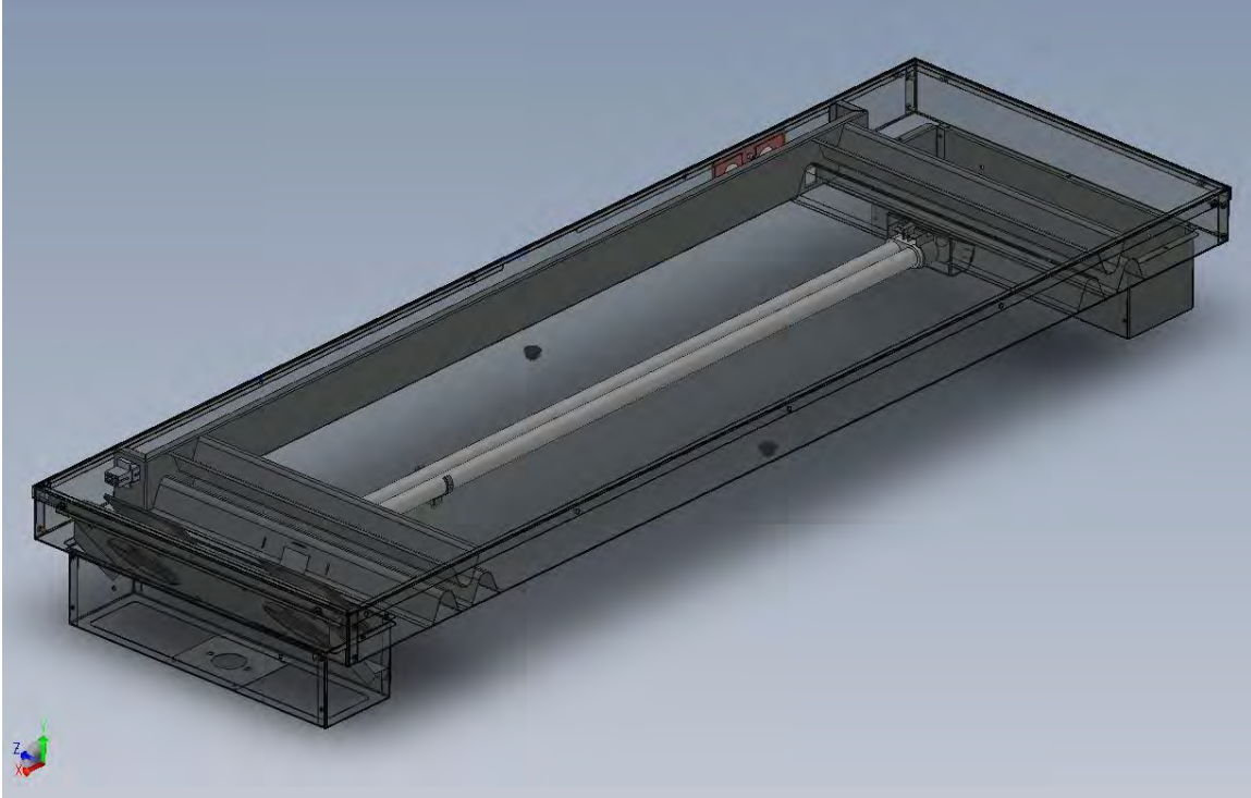
Figure 2: Schematic image of UV24 System showing internal UV lamps and irradiation chamber.
