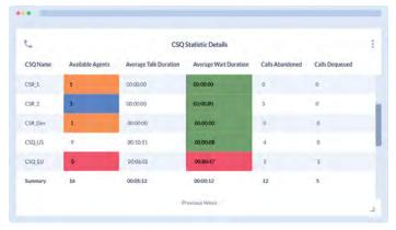
Visual alert color changes based on configurable thresholds
