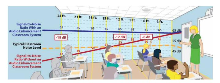
Sound technology is not about making the teacher's voice louder; it's about distributing that sound clearly and equally. At its core, the Inverse Square Law states that as the distance from a source of sound doubles, it is reduced to a quarter of its original intensity.
