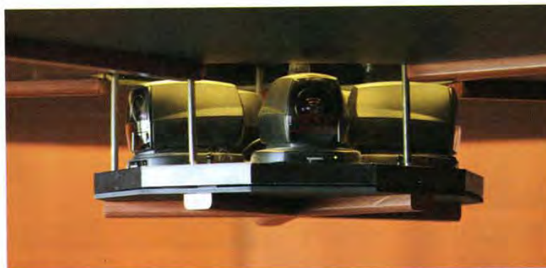
Top: Revolabs boundary mics and Altinex TNP500 Tilt 'N Plug custom pop-up laptop interfaces make for a sleek conferencing space. Bottom: A secondary lift in the center of the room holds five Tandberg WAVE II cameras, which drop down below the plasmas when needed.
